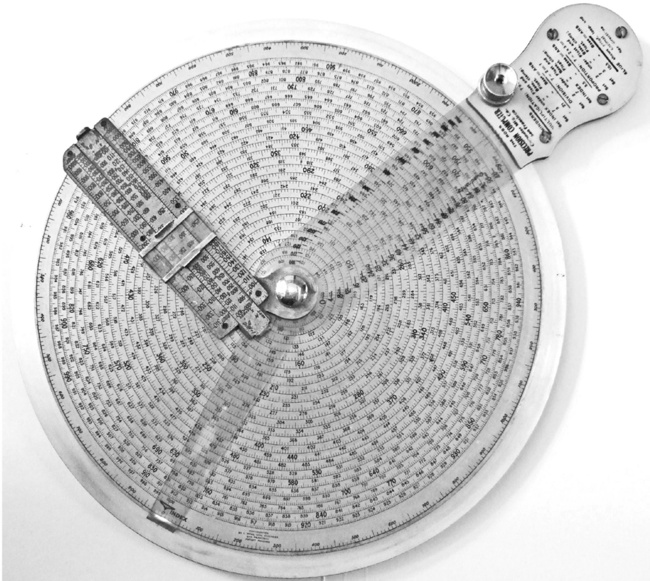
Figure 3. The Ross "Spiral" Precision Computer. Note smaller attached linear slide rule.
