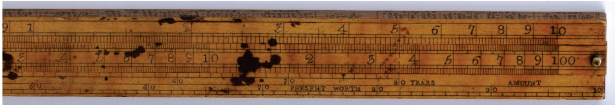
FIGURE 3b. Bevan's Engineering Slide Rule Front, Right Side
