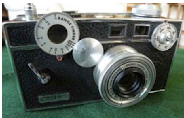
Figure 8. The Argus C-3 Camera Note that the split image range finder/distance meter on the Argus C-3 reads in logarithmic scale distances.
