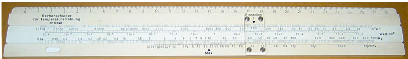
Figure 5. Front Face of the Aristo Nr. 10048 – Rechenschieber für Temperaturstrahlung from the Early 1950s
