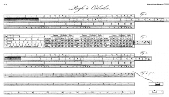
FIGURE 6. Soho type slide rule (Plate from Jomard's publication)
