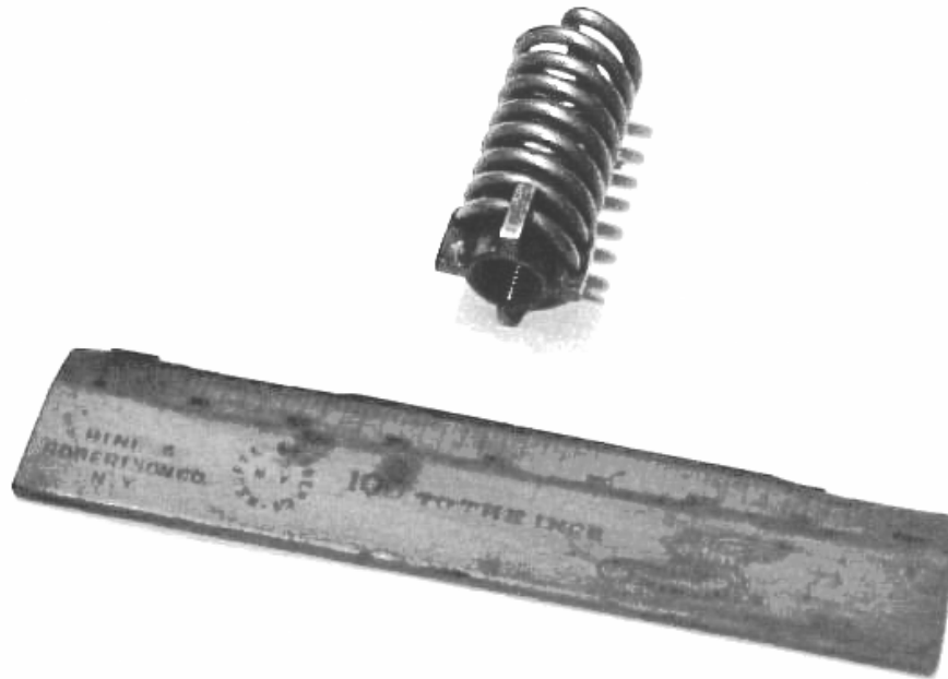
Figure 12. K&E scale and Crosby indicator spring both rated at 100 pounds to the inch.
