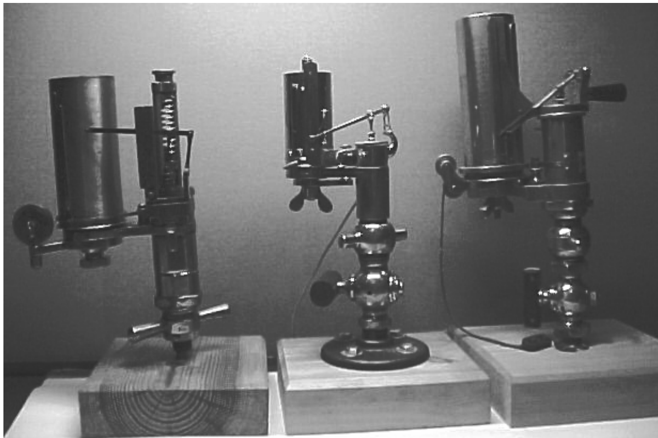
Figure 9. Three indicators that did not use Thompson's pencil movement. Left to right Tabor by Ashcroft, Lyne, and Darke.
